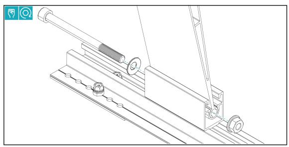
Duse the safety bolt to secure each tilt adapter to the height adapter on the starting and ending rows of an array.
