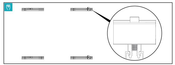
Attach end-clamps to the edge of the module field.
