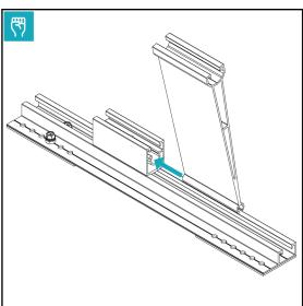
> Attach tilt adapter to ELO5 height adapter as required.
