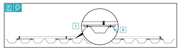
i The trapezoidal metal sheet bridge 1 is installed across two peaks. 2. The distance between the rails depends on the width of the modules and the distance between the peaks.
