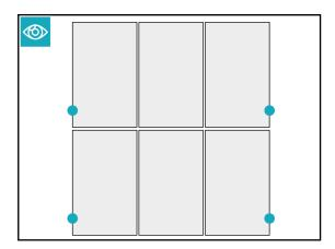
i The LSP safety bolt is attached to each back EL05 height adapter (1 x per module), where a module end clamp is mounted.
