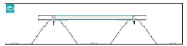
i The height adapter may only be mounted in the area between the metal screws.
