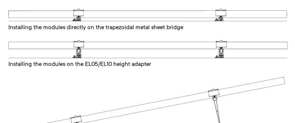
Installing the modules on the PS, PM/PL tilt adapters
