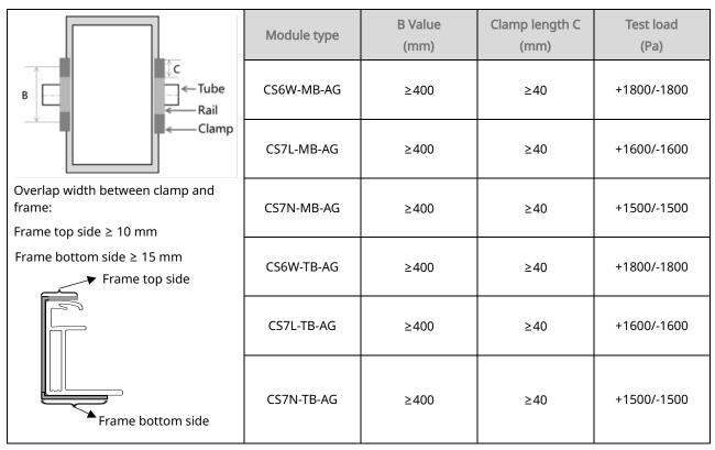
The height of the rail should be 50±10 mm.
