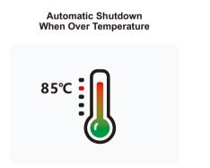
Automatically OFF the DC Power, when temperature inside of BFS-S enclosure  $\ge 85^{\circ}$ C.
