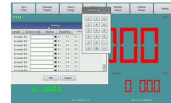
Figure 17 Communication Address Setting
