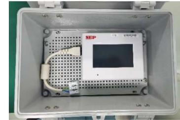
Figure 3 BDG-256 inside a weather proof outdoor enclosure
