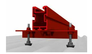
The K2 Bridge is mounted on two Hangerbolt instead of the adapter plate in order to achieve greater span widths. Depending on type, the rail is fixed to the Bridge with one or two M10x30 T-bolts.
