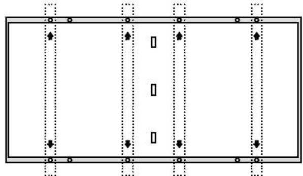
The long frame uses four outer holes (1600mm) and four holes in the center (400mm) for bolt installation
