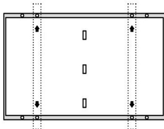
The long frame uses the inner four holes (990mm) for bolt installation
